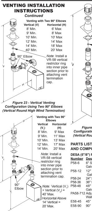
Figure 24 - Vertical Venting Configuration Using Two 90° Elbows (Vertical Round High Wind Termination) Note: Install a Firestop Plate FP-58 or a Firestop Thimble FTA-58 to maintain cleaance to combustible ceiling or insulating materials.
